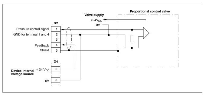
Connection of a proportional control valve without feedback
