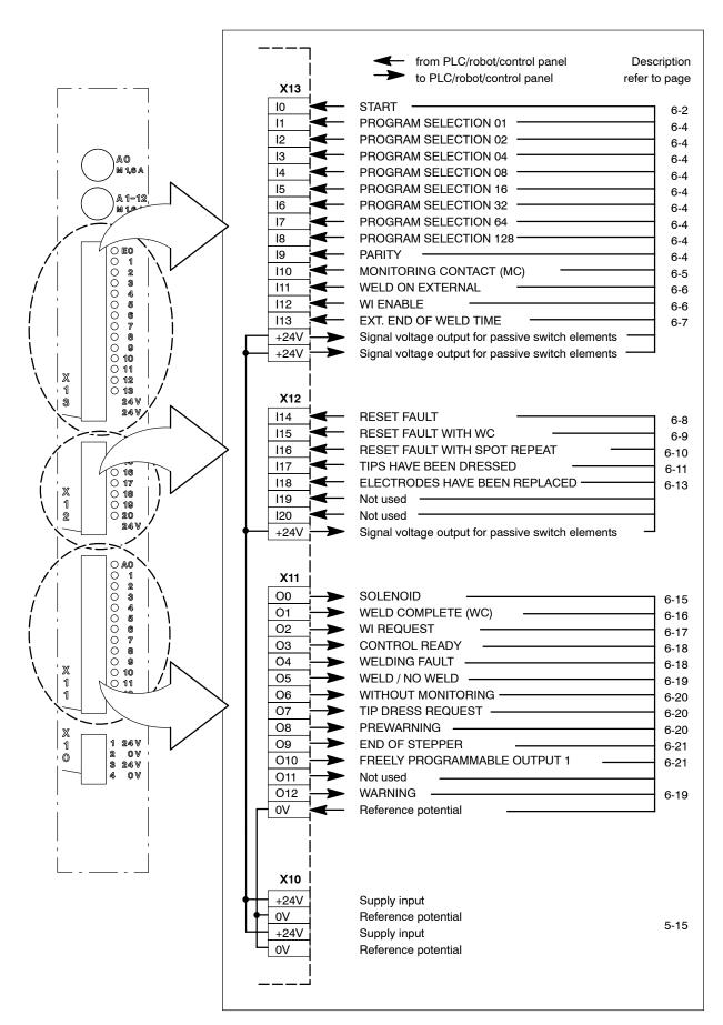
Terminal assignment of all signal in- and outputs
