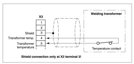
Connection for monitoring the welding transformer's temperature.
