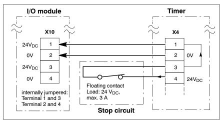
Connection of the I/O module supply to X4 of the timer
