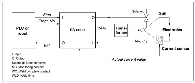
Main components of a welding station
