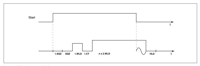
Reset of "Start" during 2.WLD in seam mode
