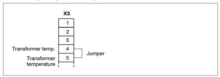
No monitoring of the welding transformer temperature by the timer
