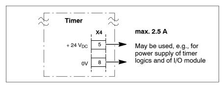
Internally generated 24  $V_{DC}$  power supply
