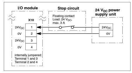
Direct connection of the I/O module supply to a separated 24  $V_{DC}$  power supply unit.
