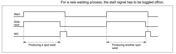
Welding operation single spot, signal sequence
