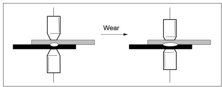
Enlargement of the contact point caused by electrode wear
