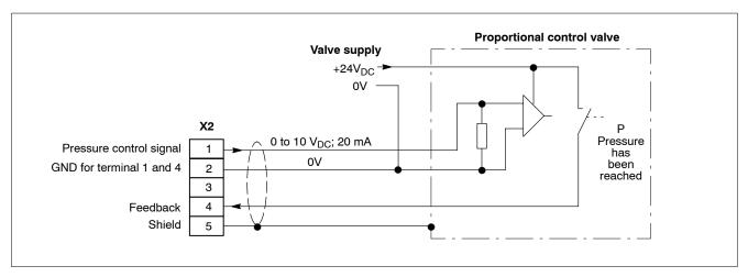
Connection of a proportional control valve with feedback
