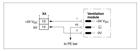
Connection of an external Bosch ventilation module
