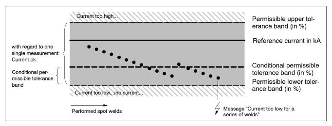
Example: Principle of the Conditional Tolerance Band with Repeat Factor = 4
