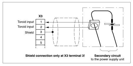
Connection of the KSR sensor on the secondary side
