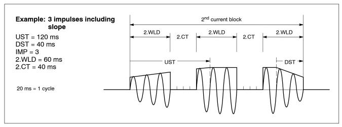
Example: Slope in connection with impulse mode
