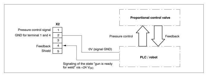
Wiring for timer types without input signal MONITORING CONTACT
