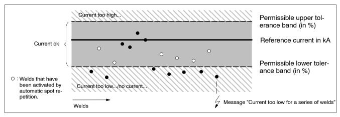
Example: Principle of the automatic spot repetition with "max. repetition" = 4
