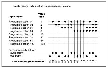
Generating the necessary parity bit
