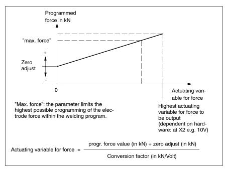
Characteristic curve for output of force value
