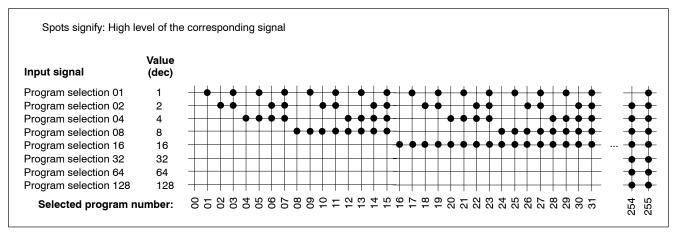
Binary coded selection of a program (of an electrode) via input signals "Program selection X"
